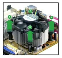
4. Remove the heatsink and fan assembly from the motherboard.
