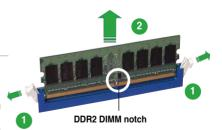
2. Remove the DIMM from the socket.
